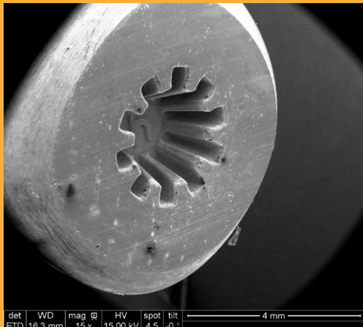
Micromanufacturing of microforging tool in tungsten carbid material by
