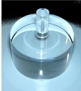
Figure 2: The Sapphire Resonator.
