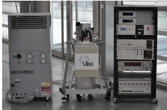
Figure 1: ULISS instrument with an air-cooled compressor, a water-cooled compressor can also be provided.
